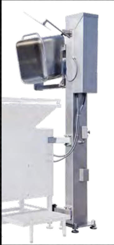
Hebe-Kipp-Beladung Lifting and tipping device
