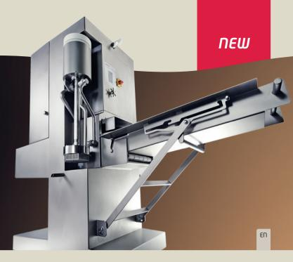
The latest curing injector on the market offers advantages that other machines cannot match. The Original IR 29 was manufactured to contemporary standards without having to compromise on traditional technologies. The result is a more accurate, extremely powerful and exceptionally efficient machine with 29 needles.
