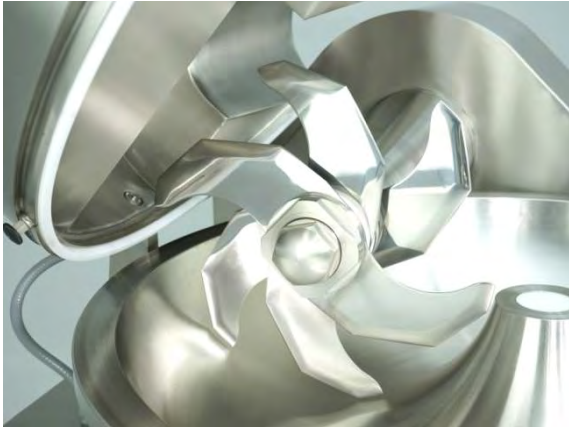
Knife Head with 6 standard knives BE-GW Steffens (Germany).
