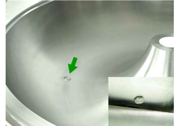
Bowl with drain plug with automatic positioning.
